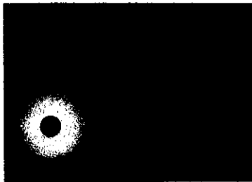
Fig. 0.9 Extra Electron Pushes Other Electrons Away, Creating 'Empty' Region in its Immediate Vicinity
